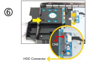
As shown, install the HDD & bracket in the chassis and push it towards the direction as indicated by the yellow arrow to connect the HDD connector (CN9).
