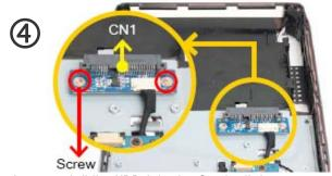
As shown, install the HDD Adapter Card with two screws and connect the cable to CN1.
