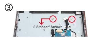
Tighten the two nuts first just as shown.
