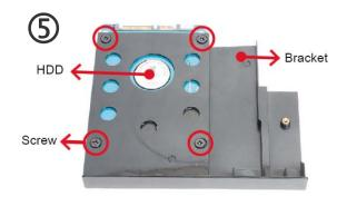
Mount HDD into the bracket with screws.
