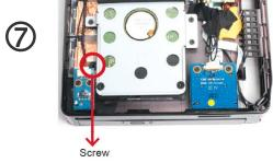
Turn your XS35 upside down and tighten the hard disk and bracket with one screw.
